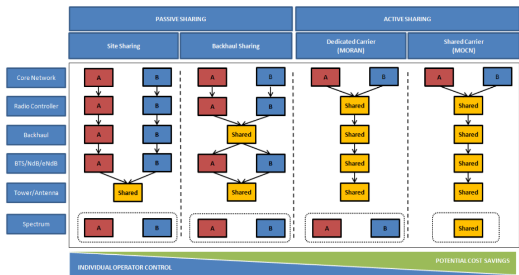
Figure 2: Mobile Network Infrastructure Sharing Source: adopted from Nokia Siemens Networks NSN
